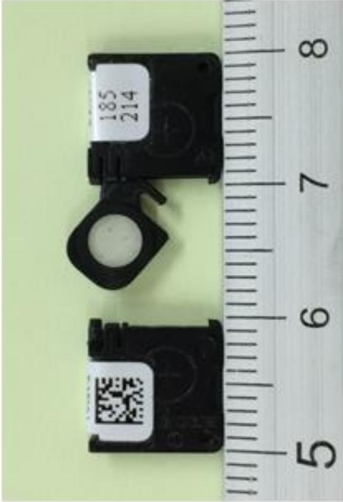
Fig 1 optically stimulated luminescent dosimeter, nanoDot
