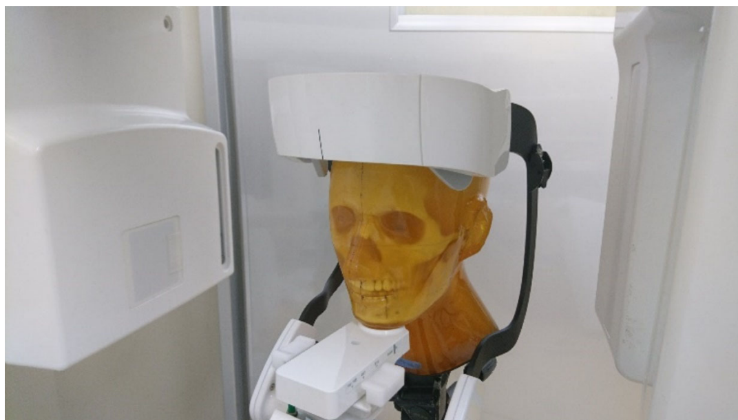
Fig 1 Urethane-enclosed skull phantom
